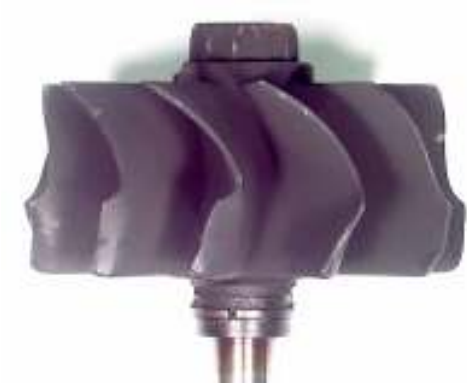
Picture 2 – Turbine wheel damage
