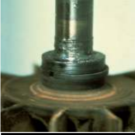
Picture 11 – Bearing damage due to hot shutdown
