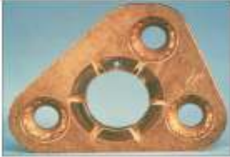
Picture 7 – Burnished and polished mating surfaces of bearings
