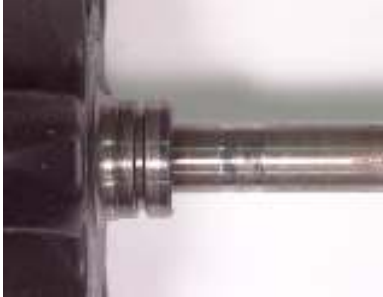
Picture 6 – Scored bearing by dirt
