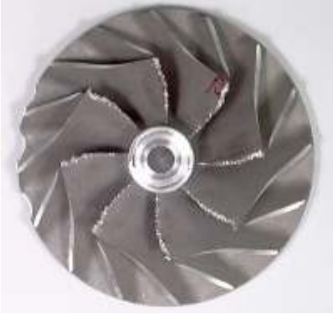
Picture 1 – Compressor wheel damage
