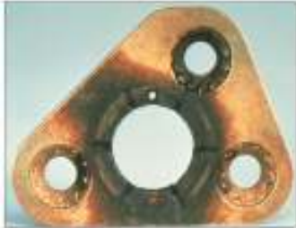
Picture 8 – Burnished mating surface of thrust bearing
