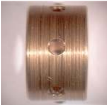
Picture 6 – Scored bearing by dirt
