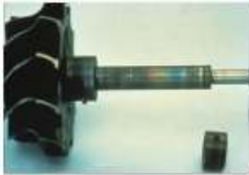
Picture 9 – Shaft burnished and discoloration - Burned journal bearing
