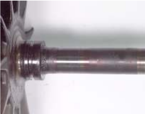
Picture 4 – Insufficient lubrication oil
